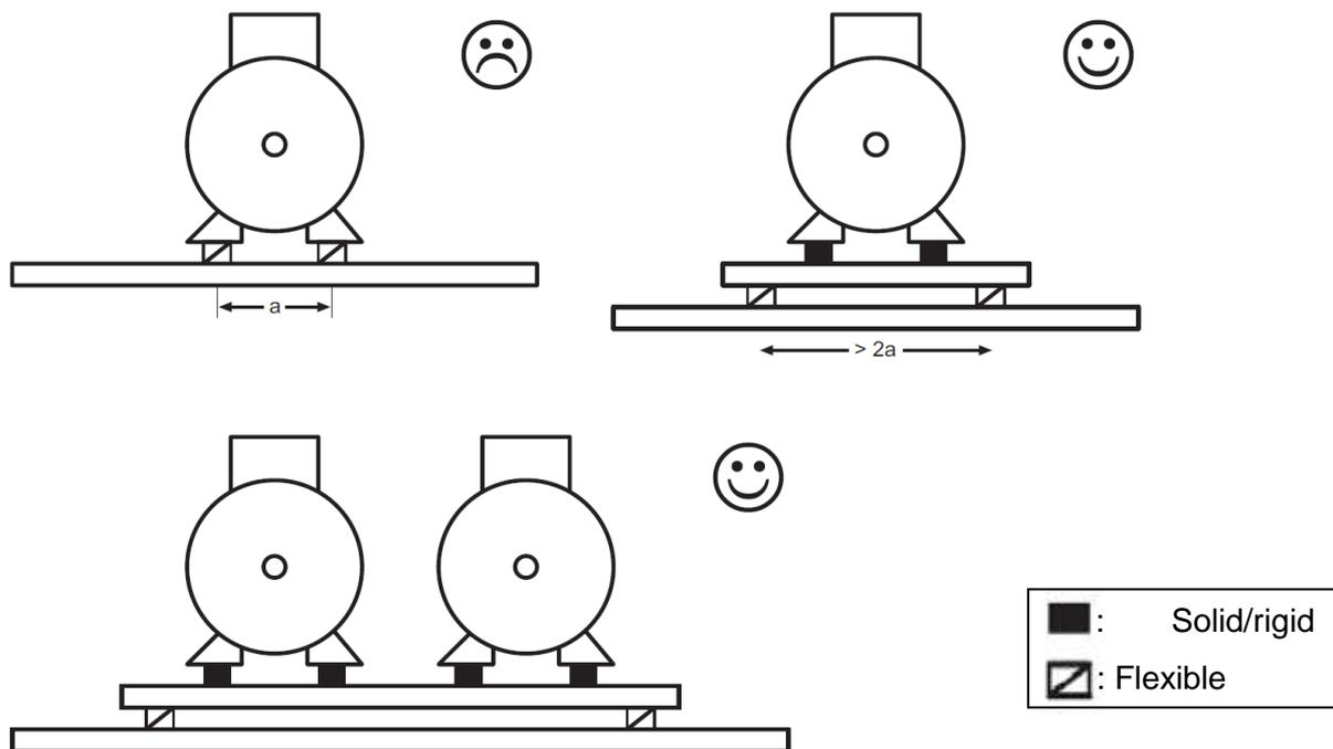
**Fig 5.3: Mounting of reciprocating compressors for variable-speed operation (Example with 2-cylinder reciprocating compressors)**
